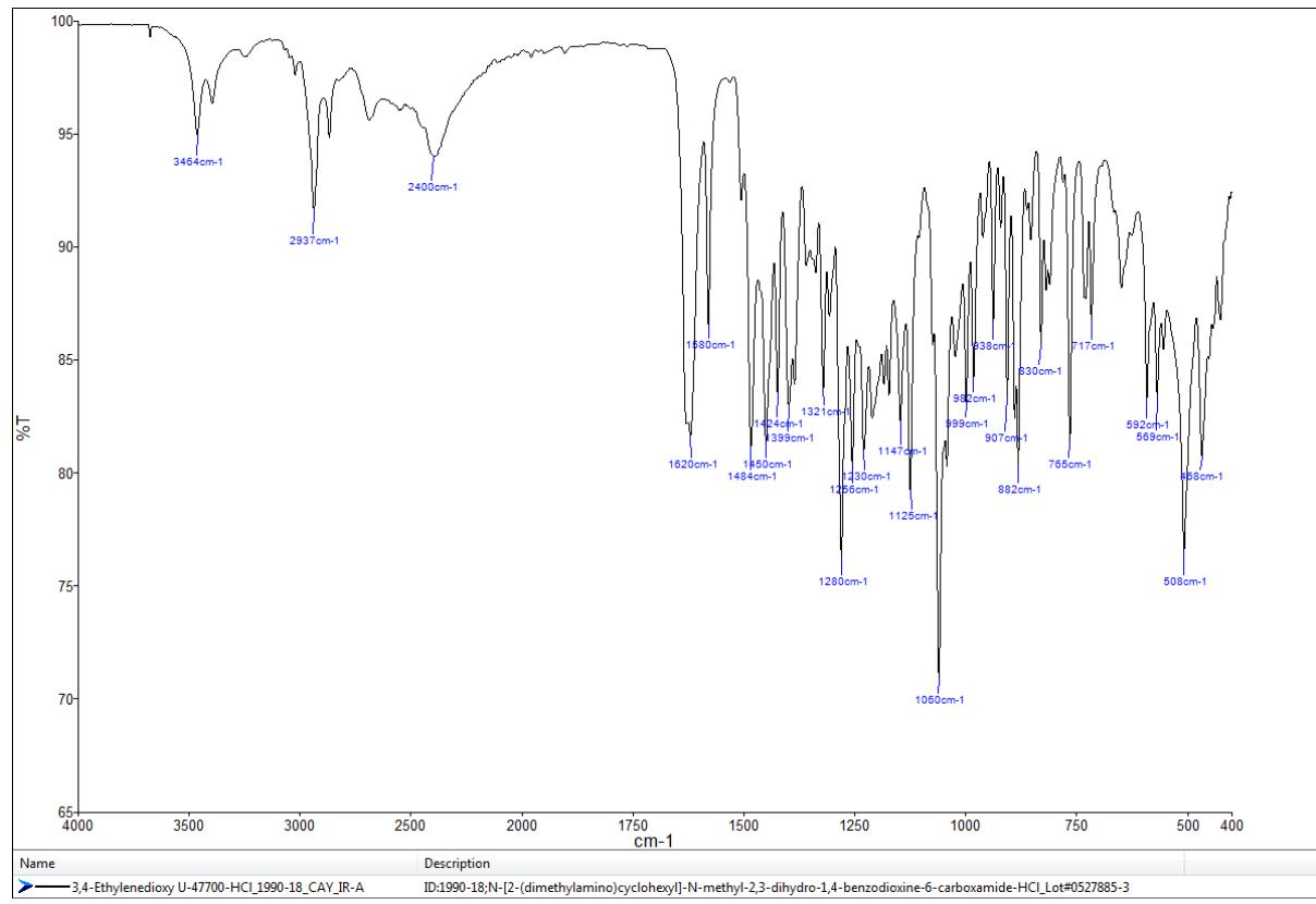
IR- (condensed (solid) phase – after chromatographic separation) - spectrum per base form
